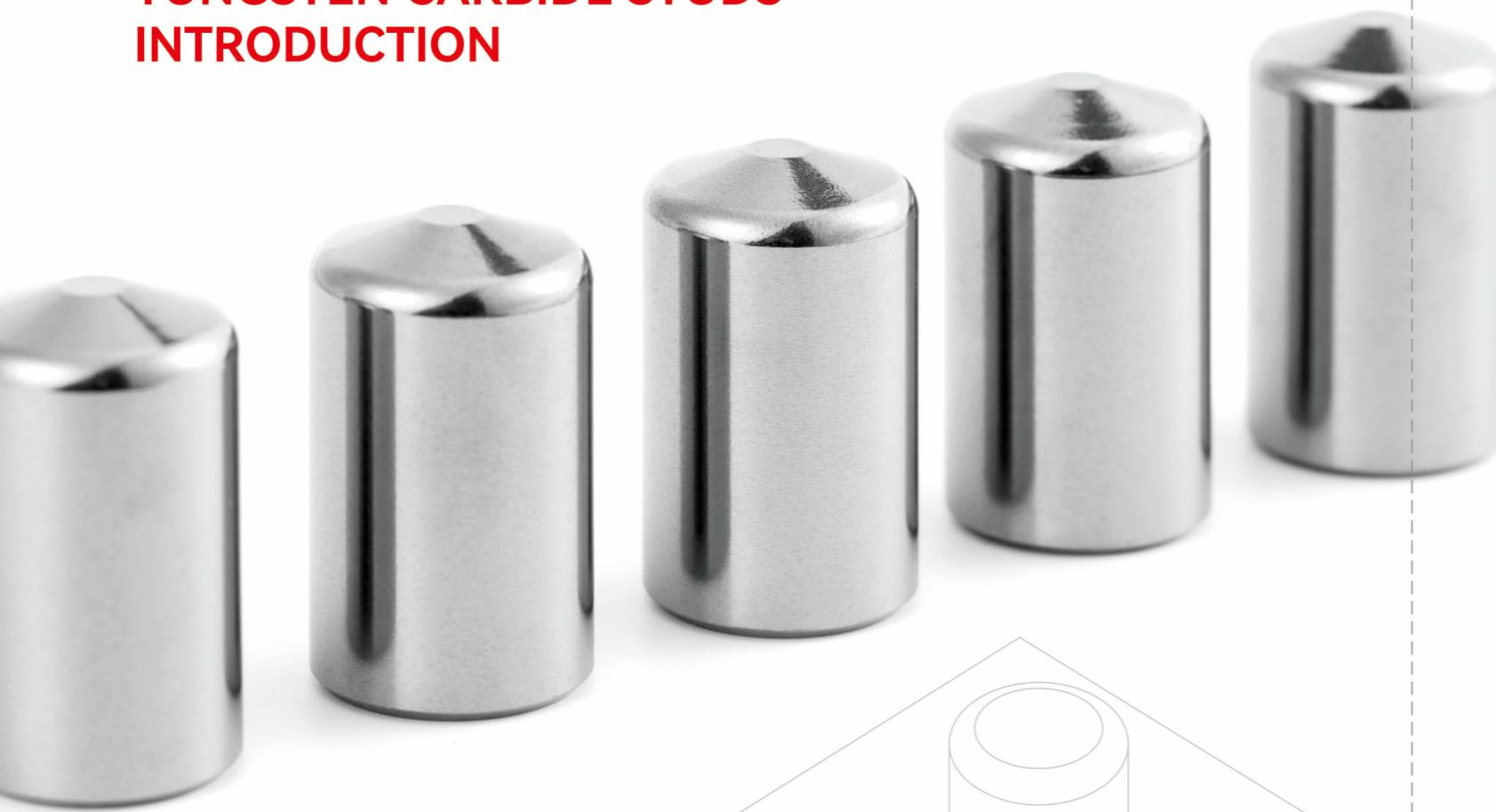
Tungsten carbide studs are core wear-resistant components of HPGR, mounted on two same size rollers surface, rollers rotate towards each other, to crush hard materials (rocks, ores, cement, coal). Protect rollers from direct wear/impact by forcing abrasion to occur on the studs, enhance roller service life and efficiency through extreme hardness (8000–20,000+ hours life time)
